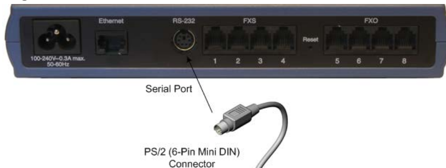
Figure 2-6: MP-11x Serial Connection with PC for CLI Communication
